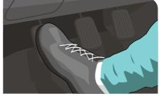
Roll on down If you're lucky enough to be parked on a hill then let the handbrake off and roll down - obviously when it's safe to do so - until the car reaches around ten miles per hour. Then let your foot off the clutch and press the accelerator pedal to make sure you don't stall.
