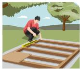
**O1** Prepare the ground You should aim to keep the shed off the ground using deck piers if possible, as standing water on the ground will be absorbed. It's also imperative that you lay the entire base of the shed on flat ground to make it easier to align the shed panels correctly.
