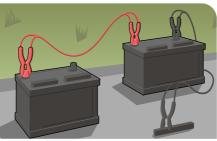
**O2** Attach the red lead to the positive terminal on the working battery and then the positive terminal on the flat one. Now connect the black lead to the working battery, but make sure the other end is attached to an earthing point on the other car and not on the battery.
