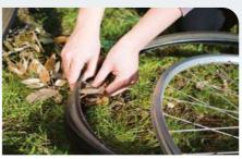
**O2 DIY, Bear Grylls-style** Collect lots of grass and leaves and pad out the tyre by filling it with the foliage – moulding them to the outer part of the tyre and working inward. You want to create a solid cushion so fill the tyre by compressing the filling and distributing it evenly around the tyre.
