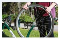
**O3** Safe and sound Reattach the tyre to the wheel – taking care that the grass/leaf mixture doesn't fall out as you do – and then fit the wheel back onto your bike. It's not an elegant solution, but it will get you home alright. To be on the safe side though, take it steady and you should be fine.
