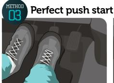
Get into gear If you don't have a battery pack or jump leads, or can't find anyone with a pair, then you're going to have to resort to the push start. Start by turning on the car's ignition, put the car into second gear and then push the clutch pedal to the floor.
