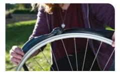
Practice makes perfect Pump some air into the tube to check for leaks - you may need a few attempts at the knot to get it just right. When it's airtight, put the tube back into the wheel. Remember it will be hard as the tube is smaller and make sure you don't inflate the tube to its usual pressure, as this is just a makeshift mend to get you home.
