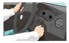
**O3** The spark of life Start the engine of the working car, leave it running for a minute and then try the ignition on the other car. If the engine starts, let it run for a couple of minutes before removing the jump leads. When you do remove them, do it in reverse order; so start with the black lead.
