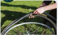
**Old Tyred out** Let's assume, for argument's sake, that you've headed out on your bike without a repair kit or a pump. Your tyre is flat and you're stuck in the middle of nowhere, so what do you do? Well, for starters, remove the wheel with the puncture and take off the tyre.
