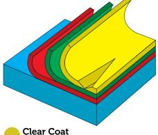
This is the first layer of paint on the car, and if a scratch has only penetrated this layer then it's moderately easy to repair. It can be just polished out with compound, but make sure to only polish the smallest area possible to avoid any respraying.
