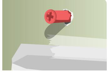
05 Plug the gap Put in the wall plugs, firstly making sure they're the correct size for the hole. If they don't go in, either use a smaller plug or a slightly larger drill bit (going up 0.5mm should do it). Attach the bracket and then repeat the same process for the other. Simple!
