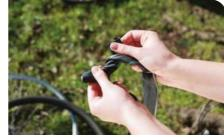
A knotty problem You now have to tie the two ends of the inner tube you have created together to form as tight a knot as possible. It's important here to keep as much slack in the tube as you possibly can, this is so you are able to get it back in the wheel – try to make sure you only use a minimum amount of the tube.
